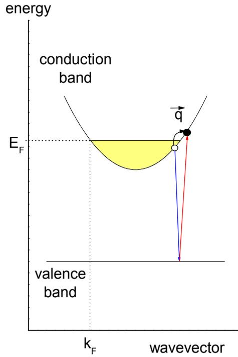
$$\omega_i = \omega_s + \omega \quad ; \quad \vec{k}_i = \vec{k}_s + \vec{q} \quad \Rightarrow \quad q \cong \frac{4\pi}{\lambda} \sin \theta \approx 10 \mu\text{m}^{-1}$$
