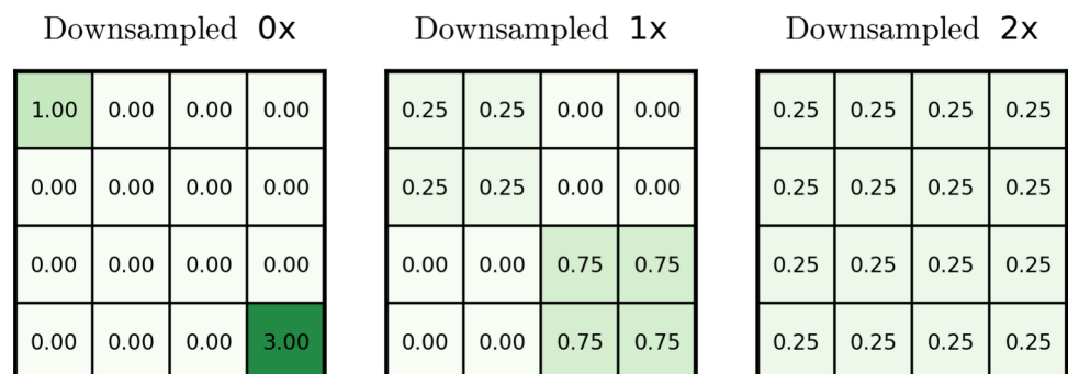
Fig. 9 Down-sampling and resizing process illustrated on 4x4 grid
