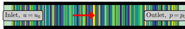
Fig. 1 Schematic of a 2D domain used in the permeability convergence test. Colors indicate local variations in porosity and permeability. In the context of Darcy-Brinkman flow, the steady solution corresponds to uniform flow. However, achieving such a solution takes place only after a (pseudo)time \tau_r due to the compressibility effects of the LBM
