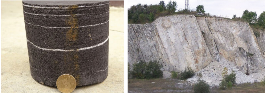
Fig. 3.21 (left) Cemented fractures in shale core (Tang et al., 2021). (right) Fractures and bedding planes in Salzgitter–Salder chalk quarry, Germany (photo by Gretarsson via Wikimedia, distributed under CC BY-SA 4.0 license)
