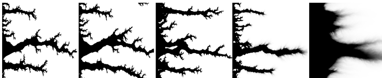
Fig. 9—The dissolution patterns in laminated fractures for \Delta = 3 at different values of the transport parameter G (Eq. 17). From left to right: G = \infty , G = 1 , G = 0.1 , G = 0.01 , and G = 0.001 .
