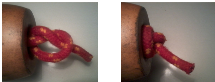
Fig. 1. Pulling the rope with a trefoil knot into the model pore (the opening of a rope float). The initial configuration (left) and the tightened configuration after a sharp tug at the rope (right).
