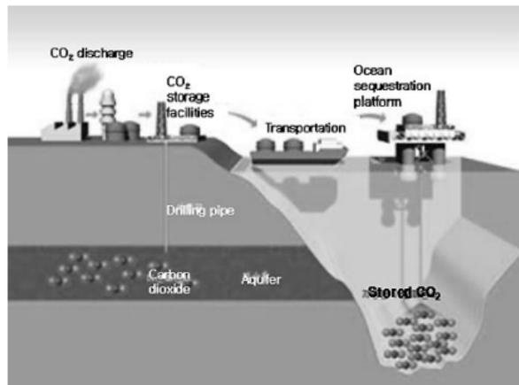
Figure: The process of injecting carbon dioxide into the earth.
