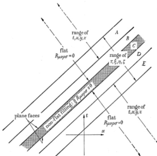
FIGURE 1. Arrangement of co-ordinate systems around sandwich wave.
