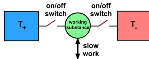
Fig. 4. Depiction of an irreversible cyclic process with a working substance (circle) using ultra-slow, pulsed heat processes through narrow low-conductivity fibers connected to hot ( $T_+$ ) and cold ( $T_-$ ) reservoirs. Either positive or negative work can be done on the working substance, which goes through a quasistatic cycle, with zero entropy change of the working substance, but non-zero net entropy increase of the reservoirs.
