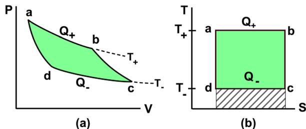
Fig. 7. Carnot cycle (CW or CCW) on (a) pressure–volume (P-V) and (b) temperature–entropy (T-S) plots for a gas working substance. Paths  $ab$  and  $cd$  are isothermal while  $bc$  and  $da$  are adiabatic. The areas  $abcd$  in (a) and (b) equal the work magnitude by or on the gas. The (shaded + hatched, hatched) areas in (b) equal  $(Q_+, Q_-)$ .
