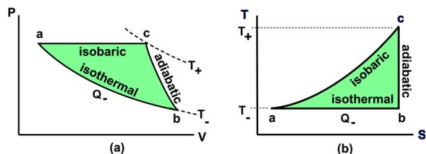
Fig. 5. (a) Pressure vs. volume for a Kelvin Cycle. (b) Temperature vs. entropy for the same cycle. Work on the system (CCW cycle) or by the system (CW cycle) is the shaded area  $abca$ .
