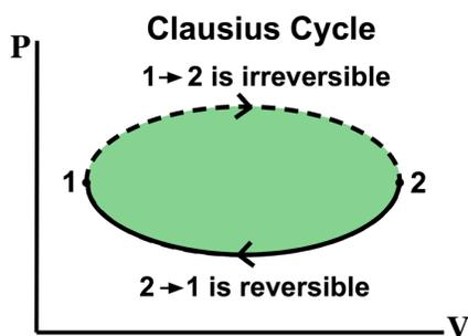
Fig. 1. Clockwise cycle with an irreversible segment  $1 \rightarrow 2$  and a reversible segment  $2 \rightarrow 1$ . The dashed line  $1 \rightarrow 2$  is purely symbolic because pressure  $P$  might not be well defined along this path, so the path cannot be graphed.
