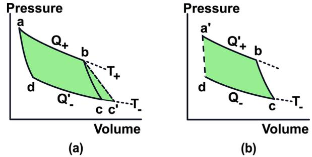
Fig. 8. Carnot cycle with (a) rapid, irreversible expansion starting in state  $b$ , leading to  $c'$  rather than  $c$ ; and (b) a rapid compression starting in state  $d$ , leading to  $a'$  rather than  $a$ . The dashed lines in (a) and (b) are symbolic, representing paths that cannot be graphed because pressure is not well defined between states  $b$  and  $c'$  and states  $d$  and  $a'$ . The latter four states are well defined.
