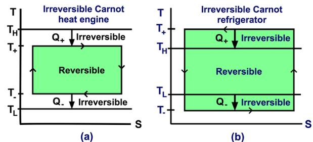
Fig. 9. Temperature–entropy plot of an irreversible-quasistatic Carnot CW (heat engine) cycle with two isothermal and two adiabatic segments. (b) Temperature–entropy plot of the irreversible CCW (refrigerator) cycle. Note:  $(T_+, T_-)$  are the working substance’s (maximum, minimum) temperatures while  $(T_H, T_L)$  are the high and low reservoir temperatures.
