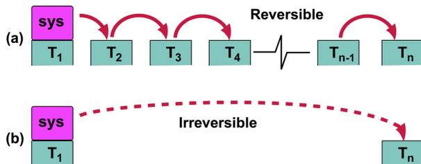
Fig. 3. (a) Heating by thermal contact with a sequence of  $n$  constant-temperature energy reservoirs, with  $T_j = T_1 + j\epsilon$ ,  $j = 0, 1, \dots, (n-1)$ . Reversibility is achieved as  $\epsilon \rightarrow 0$  and  $n \rightarrow \infty$  with  $n\epsilon$  fixed. (b) Irreversible energy transfer, bringing the system directly from the first to  $n$ th reservoir.
