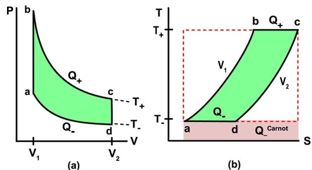
Fig. 10. Two views of the Stirling cycle with alternating constant-temperature and constant-volume segments. (a) Pressure vs. volume. (b) Temperature vs. entropy. The dashed rectangle is for a comparison Carnot cycle and the shaded lower rectangle is the energy exchanged between the gas and reservoir at  $T_-$ .
