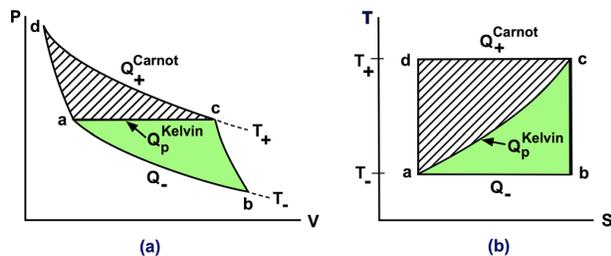
Fig. 6. Kelvin cycle  $abca$ , embedded in a reversible Carnot cycle. Note that  $Q_p^{Kelvin} = \{Q_{out}, Q_{in}\}$  for  $\{CCW, CW\}$  cycles, respectively. Subscript  $p$  connotes a constant-pressure path.
