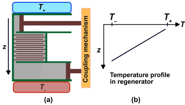
Fig. 11. (a) Depiction of Stirling cycle apparatus with regenerator in which the gas cools as the gas moves from the hot to cold side, and heats as the gas moves oppositely. (b) Temperature profile of the gas in the regenerator, regardless of gas flow direction. Adapted from D. V. Schroeder, *An Introduction to Thermal Physics* (Addison-Wesley-Longman, 1999), p. 133.
