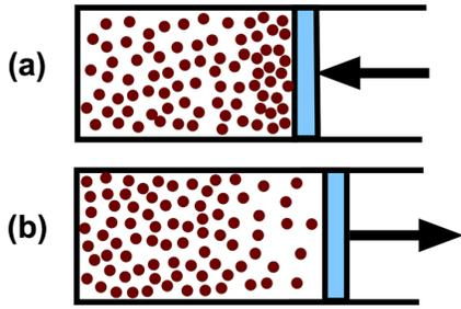
Fig. 2. Symbolic view of an irreversible quick (a) compression and (b) expansion of a gas.
