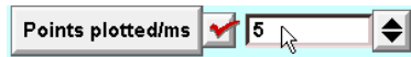
B. To keep the graph from filling up with an opaque tangle of lines, we should make sure the stored traces will be sufficiently different from each other. Plotting only 5 traces per millisecond will do the trick for this example (leave dt = 0.025 ms).
