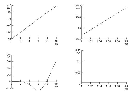
Figure 4.14. Ramp clamp using the Vector class's play() method works well with fixed  $\Delta t$  integration because command potential is effectively a continuous function of time. Top traces are membrane potential, bottom traces are clamp current.
