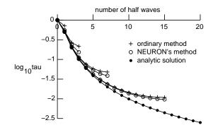
Figure 4.2. Normalized time constant for decay of spatial patterns vs. number of half waves along a uniform passive cylindrical cable (cable parameters as in Fig. 4.1).
