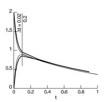
Figure 4.6. Simulation of the two compartment model of Fig. 4.4 using the backward Euler method. Left:  $\Delta t = 0.2$  s, much larger than the fast time constant. Right:  $\Delta t$  was initially 0.02 s, small enough to follow the first time constant closely. After 0.1 s,  $\Delta t$  increased to 0.2 s but the solution remained stable. Thin lines are analytic solution, thick lines are backward Euler solution. Modified from (Hines and Carnevale 1997).
