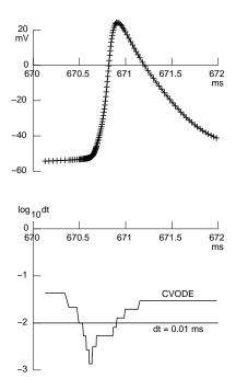
Figure 4.13. Top: An expanded view of the first spike in the second burst from Fig. 4.12. The times of computed solutions are marked by + symbols. Bottom:  $\Delta t$  fell below 0.01 ms from just before the threshold of each spike until shortly after its peak. Figure from (Hines and Carnevale 2001).
