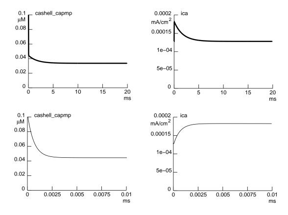
Fig. 8.3. Time course of  $Ca_{shell}$  (left) and  $I_{Ca_{pump}}$  (right) following an initialization that increased  $Ca_{shell}$  abruptly after calling init(). The traces in the top figures were thickened to make the early fast transients easier to see. The time scale of the bottom figures has been expanded to reveal the details of these fast transients. The final steady state levels of  $Ca_{shell}$  and  $I_{Ca_{pump}}$  are the same as in Fig. 8.2.
