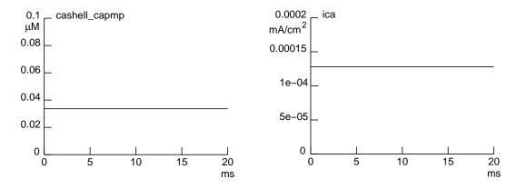
Fig. 8.2. Default initialization after setting cashell\_capmp to 0.1  $\mu M$  leaves  $Ca_{shell}$  (left) and  $I_{Ca_{pump}}$  (right) at their steady state levels of  $\sim 0.034~\mu M$  and  $\sim 1.3\times 10^{-4}~mA/cm^2,$  respectively.
