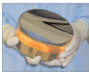
Figure 7. This photograph shows a polished and coated M4 mirror from the ETS camera. For people who appreciate ultrahigh precision, the mirror is a thing of beauty.
