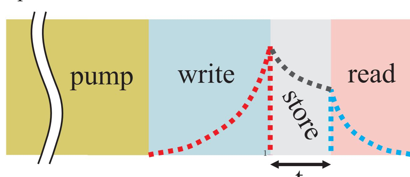
Pulse sequence starts with the optical pumping
