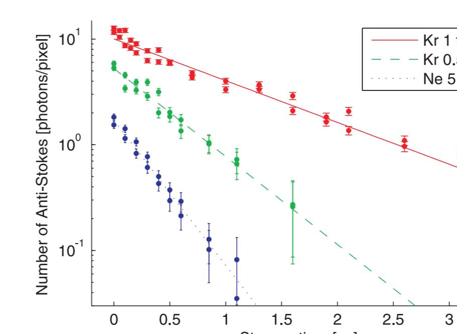
The exponential decay of the anti-Stokes scattering vs. storage time.
