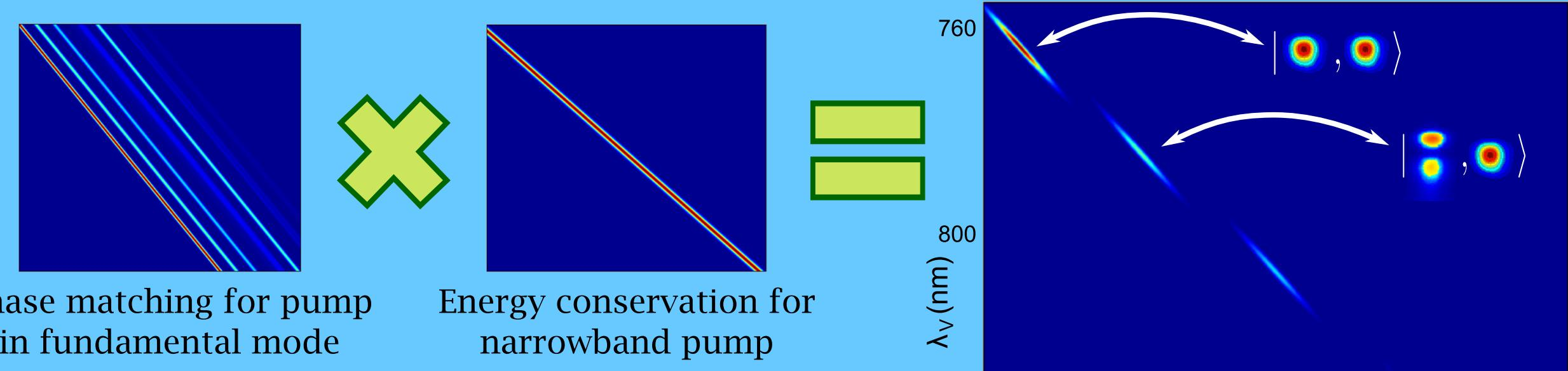
The resulting joint spectrum demonstrates distinct spectral contributions ("islands"), with the downconversion process involving 3 fundamental modes being well separated spectrally. This happens provided that the pump field is appropriately narrowband and **prepared in a pure fundamental mode**. If this is not the case, the "islands" contain multiple contributions from different modes and may spectrally overlap.
