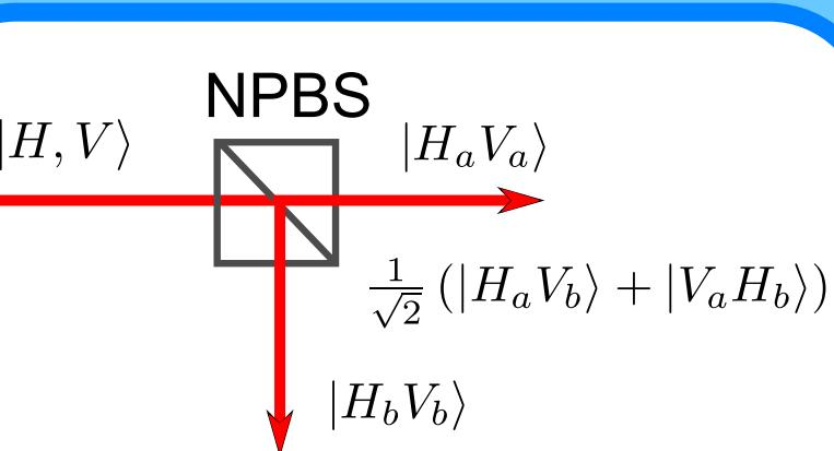
Purity of the downconverted photons can be verified by creating an entangled state conditional on detection of a photon in both output modes of a non-polarizing beamsplitter [2] (see left).
