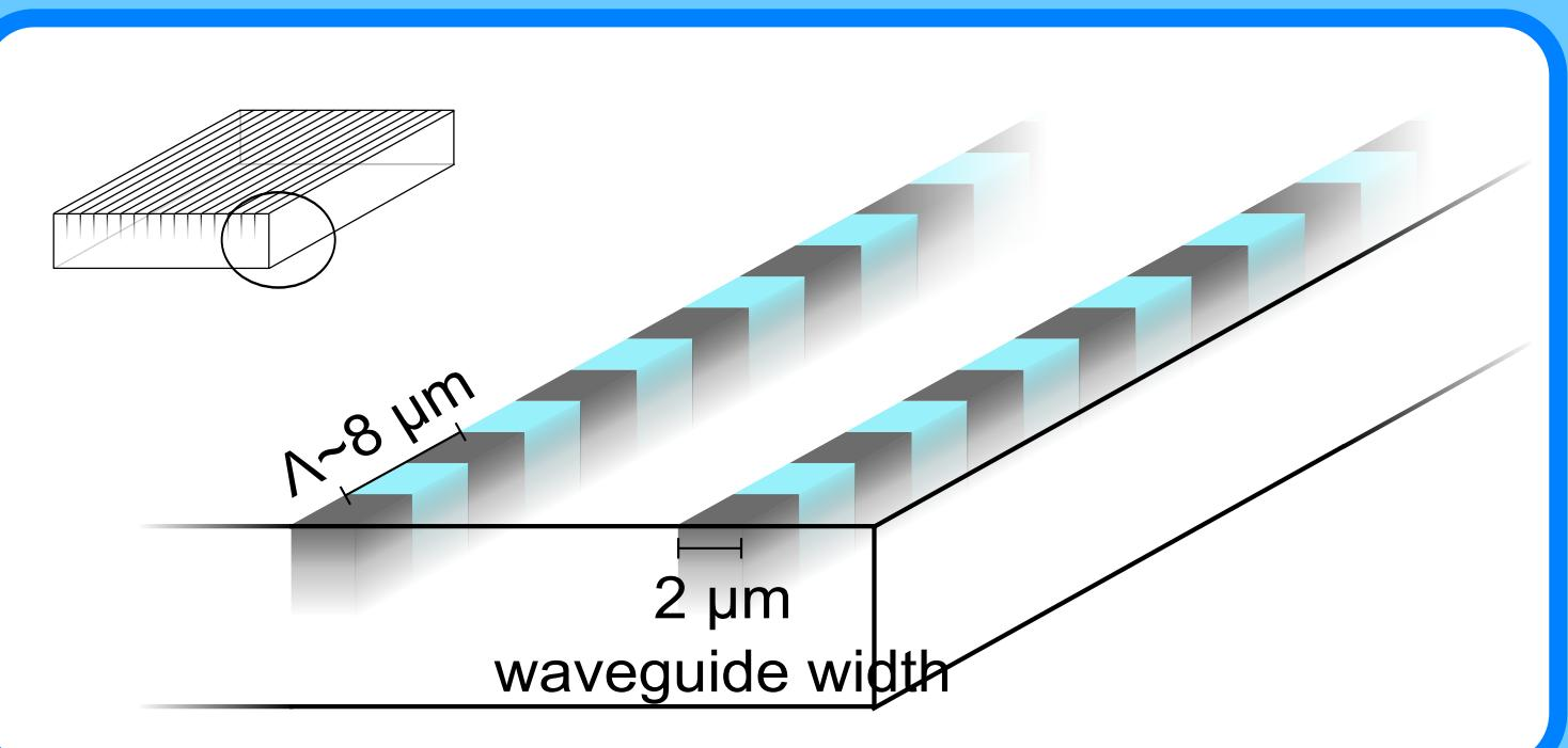
Waveguide sample characteristics. A commercially available sample: z-cut KTP crystal containing several waveguides fabricated on its surface by ion exchange. Waveguide width was 2  $\mu\text{m}$ , effective depth approx. 5  $\mu\text{m}$ . Length of the sample: 1 mm. Quasi phase matching was provided by periodic poling.
