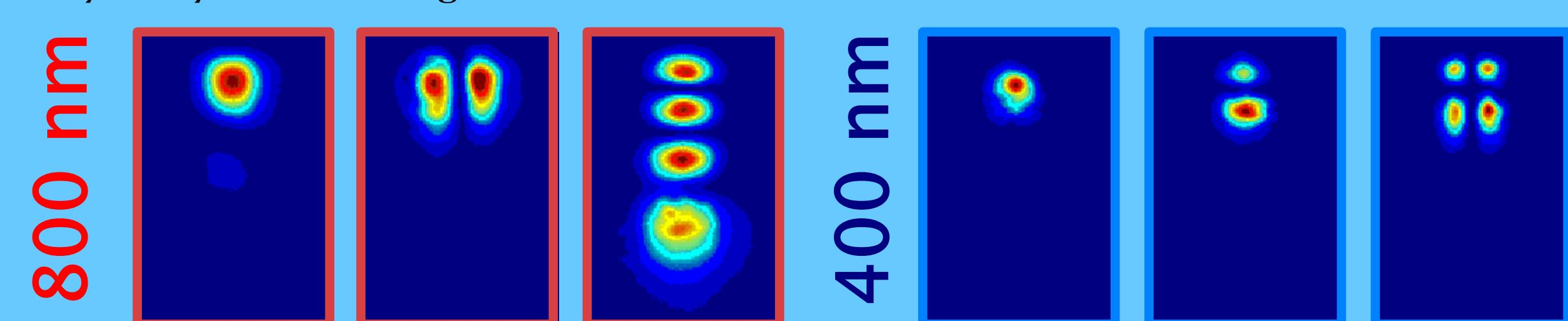
The multimode nature of the waveguide in general causes mixedness in the transverse spatial degree of freedom of downconverted photons. Whereas this can be suppressed by spatial filtering using single mode fibers, it comes at the cost of additional losses and thus significant reduction of the source efficiency. Thus arises the question of possibility to provide single mode operation of a PP-KTP waveguide based downconversion source without resorting to spatial filtering, namely:
