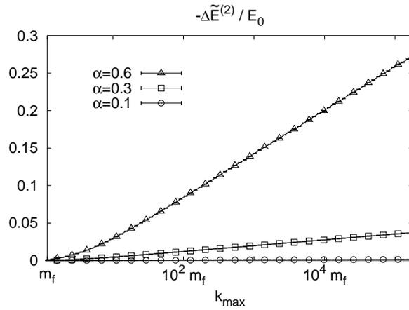
Figure 4.3: Dependence of the most singular part of the second-order correction (Eq. (4.30)) on the cutoff  $k_{max}$ . This correction diverges logarithmically for large  $k_{max}$  even for small coupling constants  $\alpha$ , though the matrix elements of the two-body Hamiltonian do not depend on  $k_{max}$  for momenta smaller than  $k_{max}$ .
