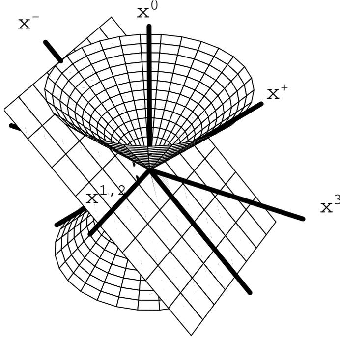
Figure 3.3: Light-front initial conditions are specified on a hyperplane  $x^+ = x^0 + x^3 = 0$  (a null-plane tangent to the light cone); dynamical evolution determines the system's state at different light-front times  $x^+$ .
