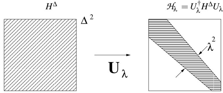
Figure 3.5: By a unitary (similarity) rotation the bare Hamiltonian  $H^\Delta$  is transformed into an effective Hamiltonian  $\mathcal{H}_\lambda$ , which is narrow (of width  $\lambda$ ), but equivalent to  $H^\Delta$  (because of an appropriate change of elements within the non-vanishing near-diagonal band).
