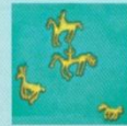
STM nanolithography image obtained by electrical local probe oxidation technique on ultrathin titanium film. Scan size 2.5x2.5 µm.
